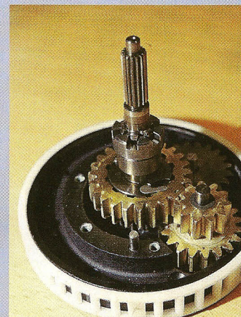
Exposed clutch system used to operate an extra two sets of gears
