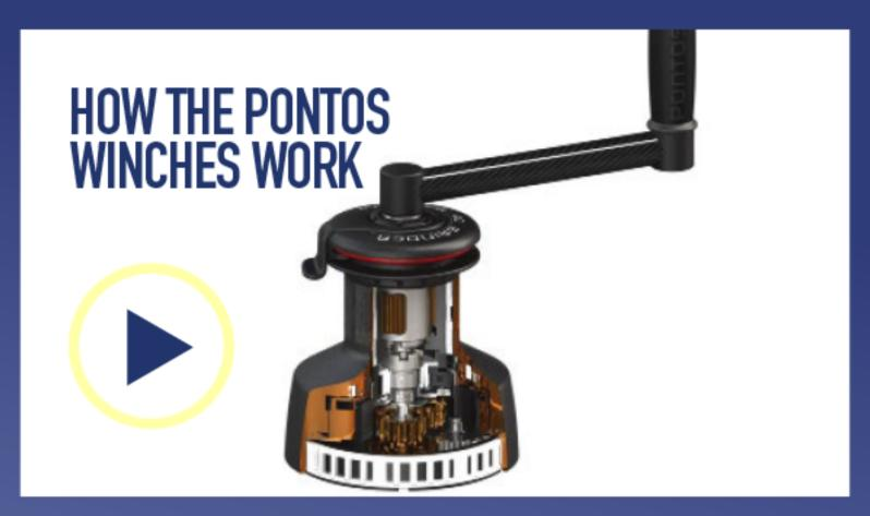
The totally mechanical system that allows, by reversing the direction of rotation of the winch, to insert the third and the fourth speed is based on a dog clutch and the mechanism that enables it to move and become engaged. The clutch movement is the key, and this is where Pontos have introduced the real innovation. When the tension on the drum increases and reaches a specific level two springs are compressed and these activate the mechanism.
